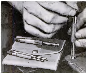
Turning a knob expands a split ball inside the hole
